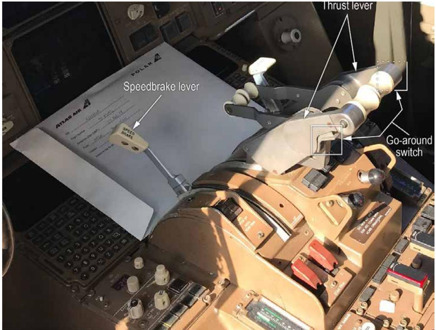
switches. The investigators observed that the airplane responded by climbing and the speedbrakes did not automatically retract. Concurrent with go-around mode activation, the flight mode annunciator at the top of each ADI display annunciated “GA/GA/GA/CMD” in green (with a temporary box around each “GA”) to indicate, respectively, that the go-around mode was active for autothrottle, pitch, and roll and that the autopilot function of the AFDS was engaged.
