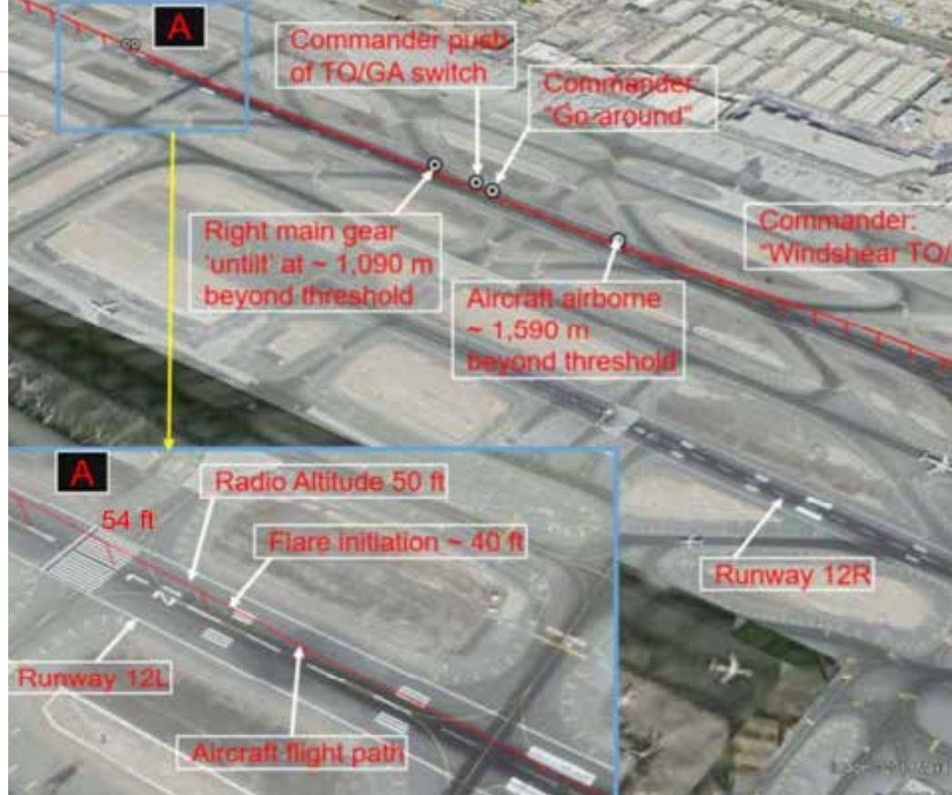
runway caused it to 'until' as indicated by the main landing gear 'tilt' and 'until' switch position recorded by the Aircraft FDR. Runway contact was made at an airspeed of 161 kt IAS, 14 kt above the landing reference speed of 147 kt. From 0837:16 to 0837:22, as recorded by the Aircraft FDR, both main landing gear experienced a series of 'tilt/until' cycles. During this six-second period, there were two automatic partial movements of the speedbrake lever recorded by the FDR.
