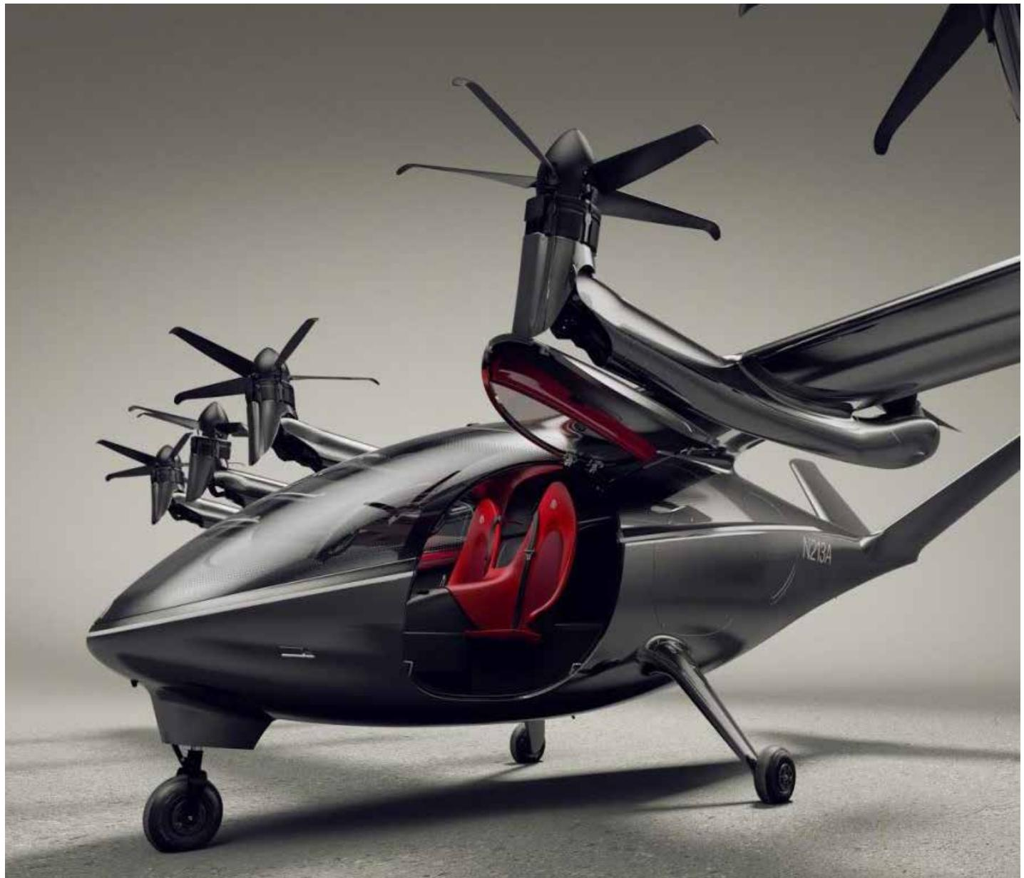
Adcock and Adam Goldstein, Archer is developing a commercially viable all-electric UAM platform that will move people throughout the world's cities in a fast, safe, sustainable, and cost-effective manner. The fully electric vertical takeoff and landing aircraft is expected to be capable of traveling distances of up to 60 miles at 150 mph using technology available today.
