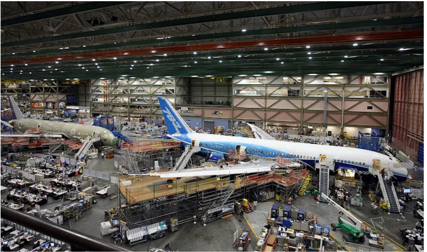
Boeing's 787 airplanes are assembled at the company's manufacturing plant in Everett, Washington, in May 2008. The 787's earliest production block, nicknamed the "terrible teens," consisted of heavily overweight, out-of-tolerance airframes that sat for years in rework because they did not meet delivery standards. KEVIN P. CASEY / BLOOMBERG / GETTY IMAGES
